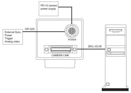
TM-6710/6710CL High-Speed Progressive Scanning CCD Camera **PULNIX**®
